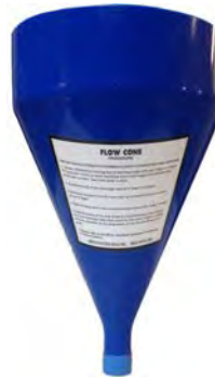
FLOW CONE TO TEST GROUT
